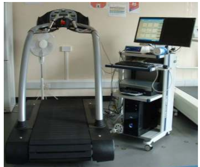
Figure 3 Experimental set up showing the treadmill and Metalyzer 3B-R2 used to record HR, \text{VO}_2/\text{kg} and the RER.
